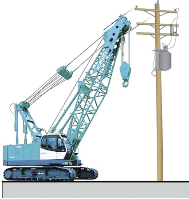
Figure 8.9 Any equipment that extends above the ground, such as cranes, booms, scaffolding, or ladders can accidentally come in contact with high-voltage lines if you do not take distance requirements into consideration.
